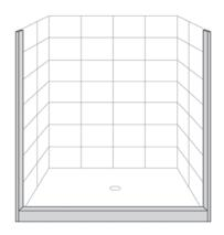
One piece curb to be cut to fit and attached on site with silicone.
