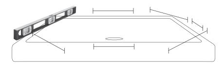
After the plumber has connected the drain, the substrate material (sheetrock, etc.) is ready to be installed. The substrate material should stop approximately 1/4" above the flange of the pan. See the diagrams below.
