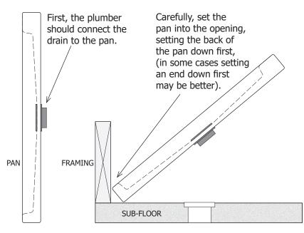
Carefully lower the pan down into place, joining the pan drain and the floor drain.
