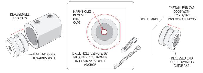
With the Guide Rail End Cap Cogs installed to the Wall Panels, you can now assemble the ROLLERS onto the GLASS DOOR. Disassemble the ROLLERS using the 3/16" Allen Wrench. Install the Top Two ROLLERS into the top two factory holes in the GLASS DOOR with the ROLLERS on the Inside of the GLASS DOOR and with the Door Handle to the Right. **Be sure to use LOCTITE Blue 243 threadlocker when installing the ROLLERS onto the GLASS DOOR.**
