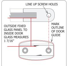
Next, you are ready to install the DOOR GUIDE. Confirm the DOOR GUIDE is set in the #12 Position by looking at the bottom. Place the DOOR GUIDE at 1 7/16" from the Outside edge of the Fixed Glass Panel to the Inside DOOR GUIDE channel, align the Right Side Screw Hole and the Fixed Glass Panel Bracket Screw Hole and Mark the outline around the DOOR GUIDE. Remove the DOOR GUIDE.
