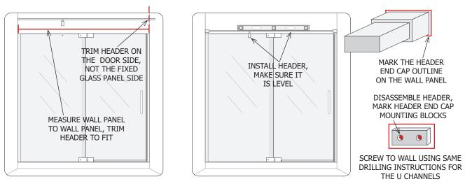
After installing the Header End Cap Mounting Blocks, re-install the Header, Slide the End Caps into place and tighten using the Allen Wrench. Next, Tighten the Header to the Fixed Glass Panel using the Flat Head Screwdriver, **do not overtighten**. You are now ready to waterproof the shower.
