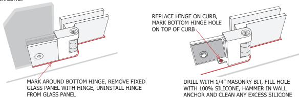
Next, Screw the Bottom Hinge onto the Shower Pan Curb. Then, Fill the bottom corner of the Fixed Glass Panel U Channel and around the base of the U Channel where it meets the Shower Pan with 100% Silicone. Next, Place the Fixed Glass Panel into the Bottom Hinge and the U Channel and Re-assemble the Bottom Hinge making sure the Fixed Glass Panel is Level. Clean any excess silicone.
