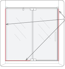
Finally, carefully run a bead of 100% Silicone both Inside and Outside the shower where the U Channels meet the Marble Wall Panels. Also, apply a bead where the Fixed Glass Panel meets the Marble Shower Pan in the Inside at the Bottom.
