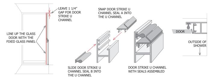
Next, hold the Door Strike U Channel up to the Wall Panel while the Glass Door is closed and even with the Fixed Glass Panel. Make sure the U Channel is Level. Mark an outline of the U Channel on the Wall Panel. Remove the U Channel and disassemble the Seals A and B. Hold the U Channel back up to the Wall Panel and Mark the holes to be drilled.
