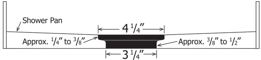
After setting the pan in place, you must check it on all four corners and diagonally in each direction for level. Shim all necessary areas to level the pan to make sure it does not move or rock at all.
