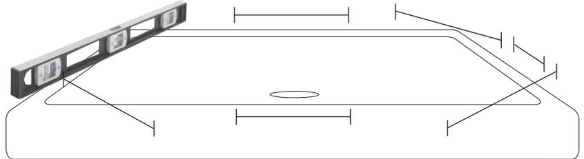
After the plumber has connected the drain, the substrate material (sheetrock, etc.) is ready to be installed. The substrate material should stop approximately 1/4" above the flange of the pan. See the diagrams below.
