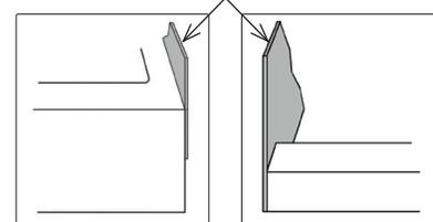
**IMPORTANT NOTE:** DO NOT lift or handle pan with either the Integral Marble Flange or the Attached Fiberglass Flange.
