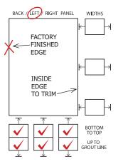
To determine what WIDTH to trim the Side Panel, measure from the PLUMB LINE that was established from the edge of the Pan or Tub back to the wall corner in all three Top, Center and Bottom locations. The OUTSIDE EDGE will be the FINISHED EDGE from the factory. The INSIDE EDGE will be the one to be trimmed, and will butt up to the Installed Back Panels.
