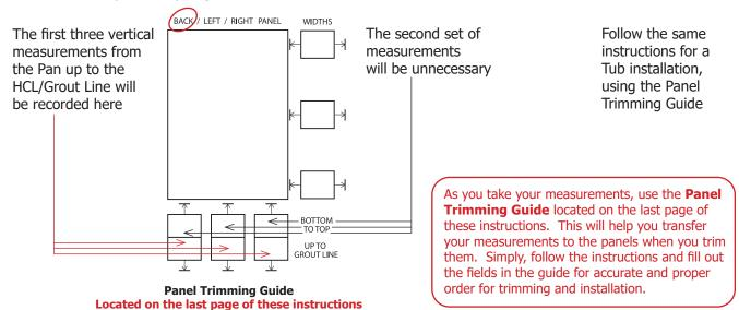
Next, measure and record the Lower Back Panel Location Width at the Top, Center and Bottom from the HCL downward towards the pan. You are now ready to transfer these measurements to the Back Panel for trimming.
