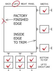
Trim the Side Panel by transferring the measurements from the Panel Trimming Guide to the Panel like before, using the Circular Saw with the Masonry Blade. **After you have trimmed the panel, thoroughly sand all cut edges with 80 grit sandpaper, especially the bottom.** Install the Side Panel using the same Adhesive Technique as the Back Panels.
