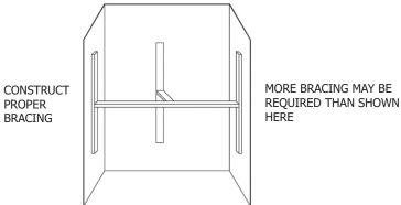
After the adhesive has had time to dry, usually 24 hours, carefully remove the bracing. You are now ready to caulk all of the joints. Use 100% Silicone where Marble meets Marble. Where Marble meets Substrate (Sheetrock, etc.) use Paintable Latex Caulk.
