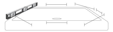
To begin with, you will want to establish a **CONTROL LINE**. This **CL** will be used throughout the installation process to make sure your panels will fit as designed. In these instructions we will be using a Tile Pattern Panel System (Product # TS-CS/12x24) as an **example panel system illustrating Horizontal Seam Back Panels first, then Vertical Seam Back Panels**.
