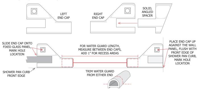
After trimming the Water Guard, drill the two holes for the Water Guard End Caps into the Shower Pan Curb with a 3/16" Masonry Bit and clean up any debris or shavings. **Fill the two holes with 100% Silicone**. Hammer in two, Green, 3/16" Plastic Anchors, clean excess silicone.
