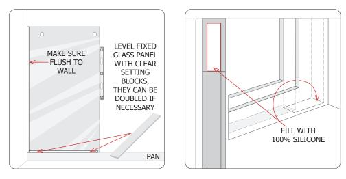
AFTER LEVELING THE FIXED GLASS PANEL AND REMOVING IT, FILL THE CORNER AREA WHERE THE BOTTOM U CHANNEL AND THE VERTICAL U CHANNEL MEET WITH 100% SILICONE.
