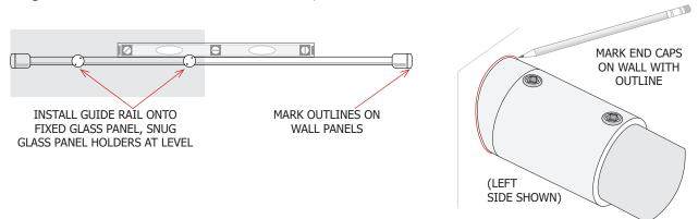
After you have marked where the Guide Rail End Caps are located on the Wall Panels, disassemble End Caps. Hold Angled End Cap Extensions back in place on the wall and Mark the inside holes, where you will drill. Drill End Cap mounting holes into Wall Panels using 5/16" Masonry Bit, Hammer in Clear 5/16" Wall Anchors and
