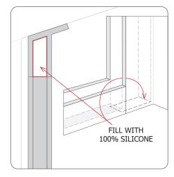
AFTER LEVELING THE FIXED GLASS PANEL AND REMOVING IT, FILL THE CORNER AREA WHERE THE BOTTOM U CHANNEL AND THE VERTICAL U CHANNEL MEET WITH 100% SILICONE.
