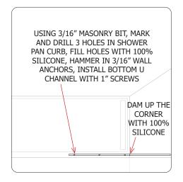
After installing the VERTICAL and BOTTOM U CHANNELS, dam up the Bottom Corner Seam with 100% Silicone.
